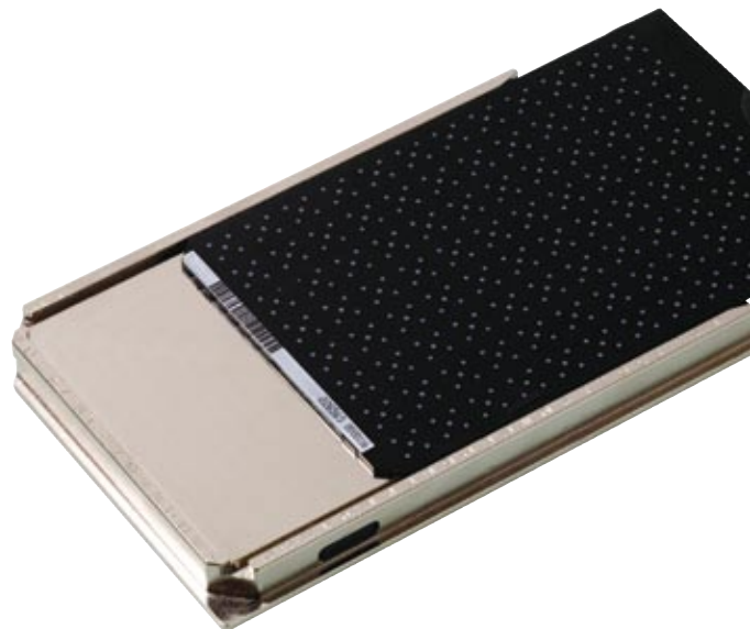
Fig. 2: The Prespotted AnchorChip. 384 anchor spots covered with HCCA matrix and 96 calibrants are prespotted.
